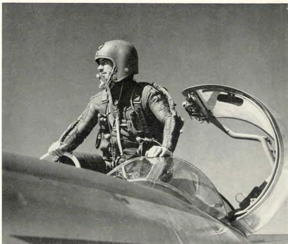
A downward ejection seat makes for a manual canopy that weighs one-fourth of power models.
