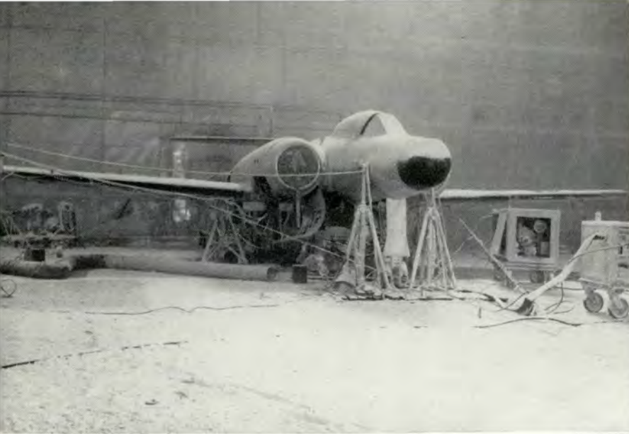
The "deep-freeze oven" cold-soaks the aircraft, then many tests including actual firing of guns are performed.
