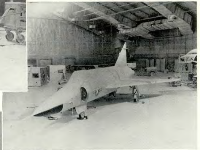
The "deep-freeze oven" cold-soaks the aircraft, then many tests including actual firing of guns are performed.
